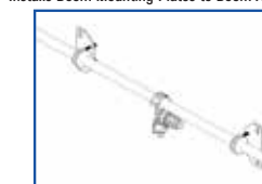
Installs Boom Mounting Plates to Boom Assembly
