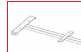
Attaches Axle Bracket to Frame Spine
