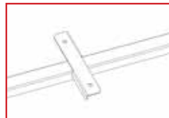
Attaches Front Tank Mount to Frame Spine
