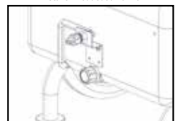
Installs Broadcast Nozzle
