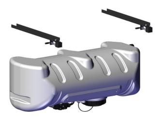
**Step 1**) Flip Sprayer Tank over to access the holes on the bottom. Position ATV mounts over Sprayer Tank holes. Attach ATV Mounts to Sprayer Tank with ½" Bolts and Washers using socket wrench. Do not over tighten.
