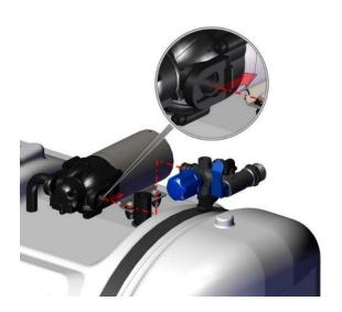
**Step 7**) Slide the Locking Clip on the Pump into the 'open' position. Insert the Regulator Assembly (PN 34-140118) into the Pump Outlet, making sure it is fully seated. Slide the Locking Clip into the 'locked' position to secure.
