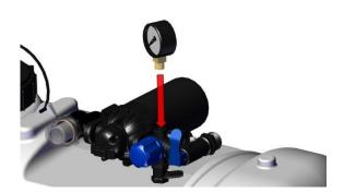
**Step 9**) Wrap a small amount of Teflon tape around the threads of the Pressure Gauge. Thread Pressure Gauge into the top of the Pressure Regulator Assembly. Take care not to cross-thread the Pressure Gauge. Note: Pressure Gauge should be facing forward with Regulator Assembly knob.
