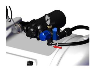
**Step 10**) Slip the ½" Hose Clamp over the end of the Spray Gun Hose. Push Spray Gun Hose onto the bottom hose barb of the Pressure Regulator Assembly. Tighten the Hose Clamp with Pliers.
