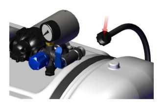
**Step 13**) Locate Boom Hose and make sure there is a Washer in the end of Boom Cap. Thread the Boom Hose to the Shut-Off Valve. Note: Use a knife to cut zip tie from Boom Assembly to free the Boom Hose.
