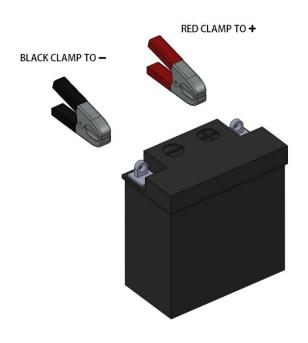
**Figure 5** Attach Wiring Harness to ATV battery as shown.
