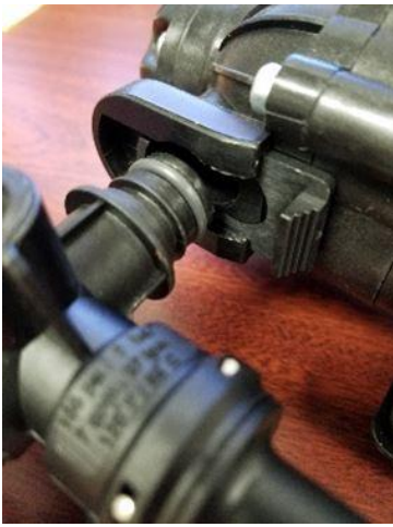
Figure 7 Insert Regulator Valve Assembly into Pump Outlet making sure it is fully seated.
