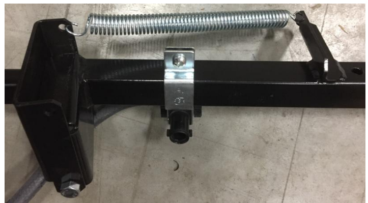
Figure 12 Attach the springs to the holes in the Hinge. Use a pliers if necessary.
