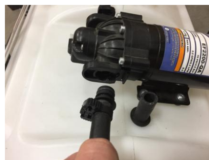
Figure 3 Remove Spray Gun Fitting from pump. Remove Fitting from Hose and discard.
