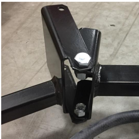
Figure 11 Position the Hinge over the holes in the Center Boom Section and secure bolts through holes with lock nuts. Do not overtighten so the hinges can swing.
