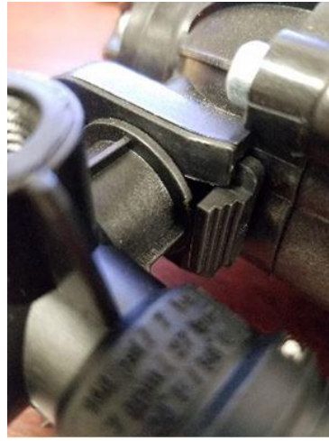
Figure 8 Slide the Locking Clip into the locked position as shown.
