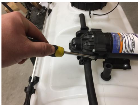
Figure 2 Use a flat blade screwdriver to push the Locking Clip back and release the Fitting.
