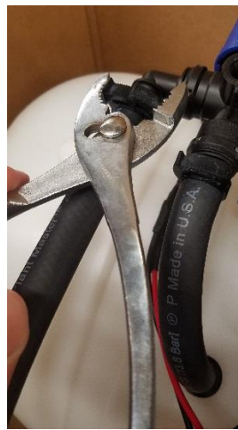
Figure 2 Use a slip joint pliers to tighten hose clamp(SHC-H) to prevent hose from shooting off during operation
