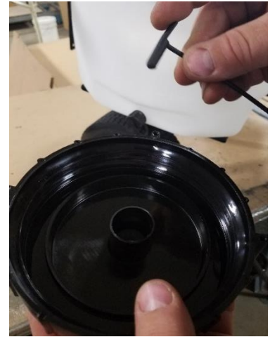
Figure 9 Attach tank lid tether to tank lid by sliding "T" end through the tank hole.
