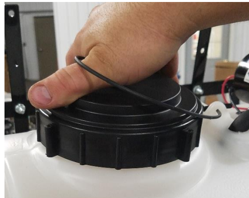
Figure 13 Screw tank lid onto tank as shown
