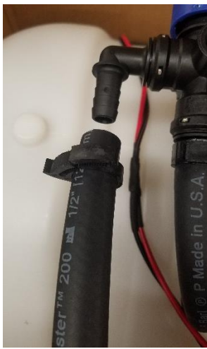
Figure 1 Attach Spray wand hose to 1/2" elbow on regulator with hose clamp(SHC-H)
