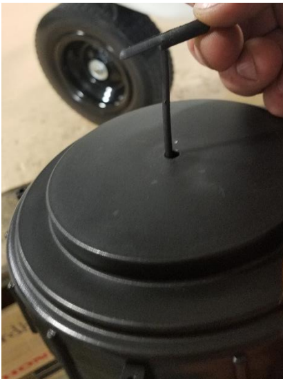
Figure 10 Tank lid tether should look like this when slid through tank lid
