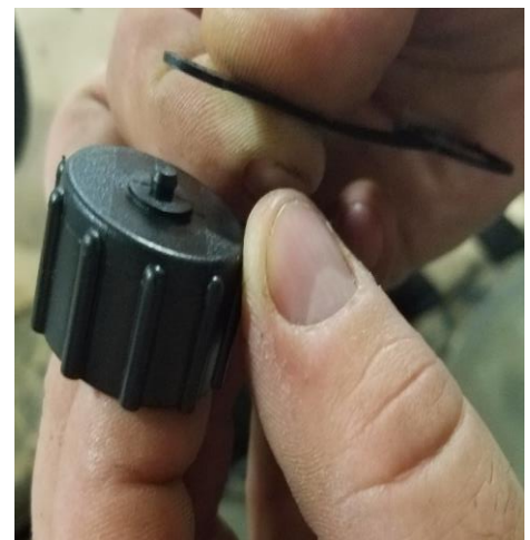
Figure 6 Push cap tether onto drain cap (33-103218)
