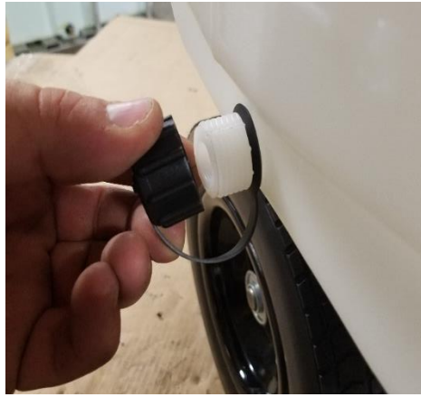
Figure 8 Attach drain cap onto tank outlet as shown. Make sure tether is on first before screwing cap on.
