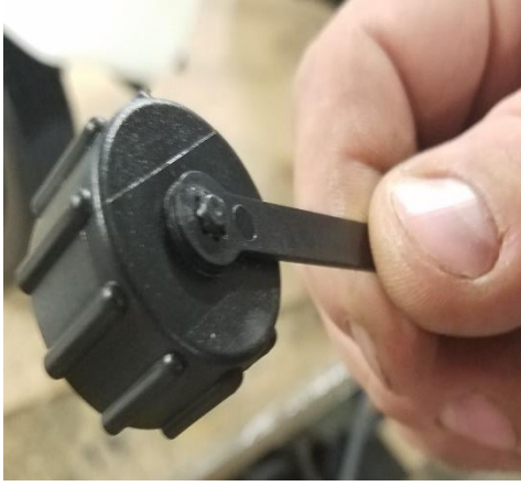
Figure 7 Drain cap should look like this with tether attached
