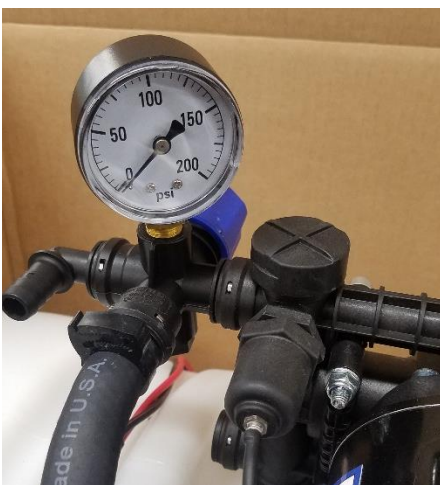
Figure 4 Screw gauge into gauge port BE SURE NOT TO OVER TIGHTEN!!! Gauge should be facing you during operation.
