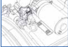
Connects Boom Assembly to Shut-Off Valve
