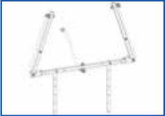
Attaches Boom Uprights to Boom Assembly
