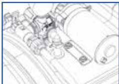
Connects Boom Assembly to Shut-Off Valve
