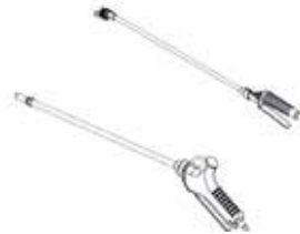
Spray Gun Assembly (1) SG-4507F or SG-2218-18
