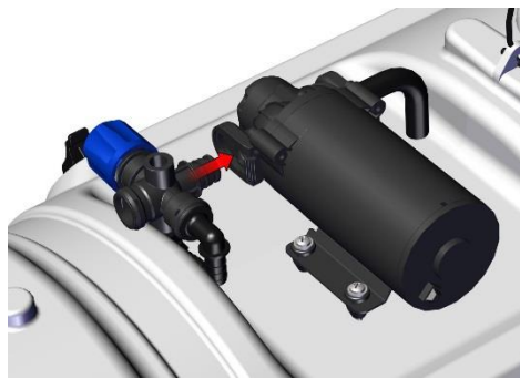
Figure 2 Locate Regulator Valve Assembly and insert into Pump port.
