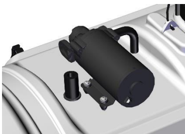
Figure 4 Drill a 3/4" hole on the mark, and insert the Top Hat Grommet and Return Hose.
