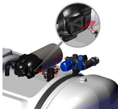
Figure 5 Reinsert the Regulator Valve into the Pump.
