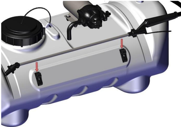
Figure 1 Check inside Tank for any foreign objects. Install Gun Clips with provided screws.
